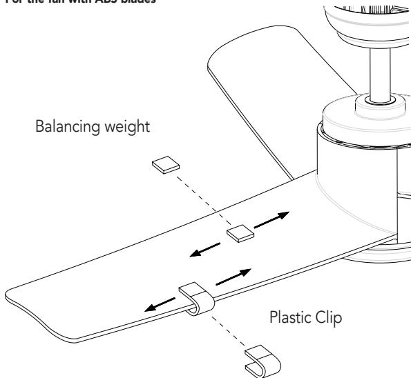
Turn on the fan and set the speed (usually high speed) that causes the worst oscillation. Turn the fan off. Remove one blade and place a balancing clip on it. Turn the fan back on and observe whether the oscillation has improved or worsened.
